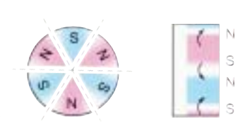
Multipole oriented in segments on one face
